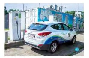
A car can drive 100 km on 1 kg H2, while a bus can drive the same distance on 7-8 kg H2 Both typically travel 400-500 km before they need to refuel. A fuel cell car usually has a 5 kg tank at 700 bar, while a bus tank holds 35 kg H2 at 350 bar
