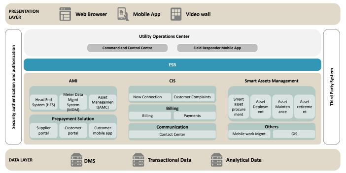
**Functional & Presentation layer:** This layer provides easy access to utility operations center users and field staff through web, mobile or video wall interfaces. Users have flexibility to customize the views to suit their needs
