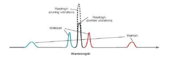
Brillouin Scattering is prominent in case of Strain signals predominantly and in some cases for temperature signals. Brillouin Scattering varies due to changes in the reflective index within the fibre and is setup as a loop (2 cores within one cable). The increase or decrease in reflective index can be due to strain or temperature. Special techniques are used to separate the two to give independent readings for temperature and strain.
