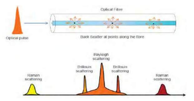
Rayleigh backscattering is prominent in case of Acoustic, Sound and Vibration signals near the fiber optic sensor. Increases and decreases in the in the Rayleigh component of the backscatter can be attributed to density variations due to vibration of the fibre. These changes in density variations can be measured and reported as Sound, Vibration or an Acoustic wave form.
