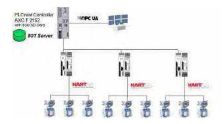
One controller OPC UA integrated can handle up to five full extended HART Gateways with 40 connected sensors = 200 sensors in sum.
