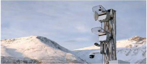
The two avalanche radars with thermal and PTZ cameras and communication devices.
