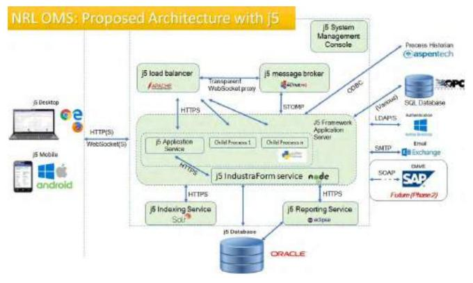
Figure 2. represents the proposed architecture of NRL OMS with j5.
