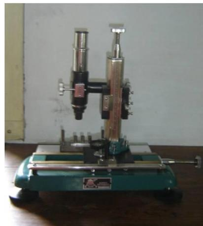
**Fig: 11** Traveling Microscope
