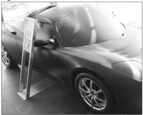
Inside were a couple of non-functional but historic Teslas: The flat-black Aero Buck, (*above*) which was computer-machined from solid fiberboard from the scans of the original clay model, and used for wind tunnel testing, and the hand-built "Drivetrain Mule," the second engineering vehicle built by the company and the first to resemble the Roadster's final design.
