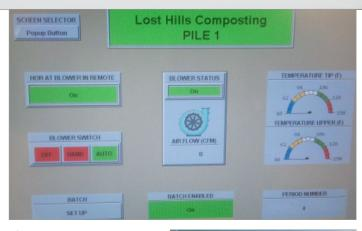
The MOR's AM/HMI provides compost facility owners/operators continuous monitoring, more historical composting data logging (every five minutes) and storage (up to 90 days), accurate data for improved process management and control, and resultant lower operator time and costs.
