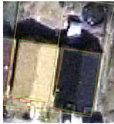
Figure 6. Discrepancy between manually digitized residential buildings. (Green)—digitizing on a full image; (red)—digitizing on parcel-sized images
