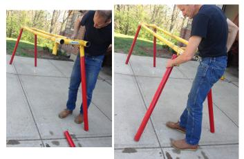
Step 6. The middle leg sections are next. The left side section will have a winch on the top, make sure the winch handle is facing out.
