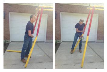
Step 8. Unwind the winch giving you slack on the snatch blocks and end hook. Attach the end hook onto the internal eyebolt on the shoulder, then attach the internal snatch block hook onto the external eyebolt on the shoulder unit. Do this for both winches on each end.
