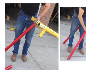
Step 5. Insert the red top leg sections on the opposite side of the cross brace assembly.
