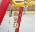
Step 9. Now insert the bottom leg segments making sure that the eyebolts on the bottom are facing inward so that tension chains can be attached. For this step, two people are needed, one to hold the unit up, the other to insert the bottom leg segments.
