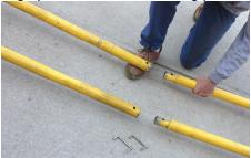
Insert locking pins with bend up, once in rotate down. To remove, rotate bend up and pull out.
