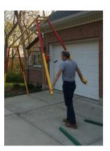
Step 10. The unit is now assembled and is ready to attach the tension chain between the four legs. The tension chain has three pieces. Two separate chain loops with two quick links that attach to the eyebolts on the bottom of the leg.
