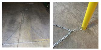
The two chain loops, now attached to the legs, pull the middle chain sections towards each other and attach the third chain segment, using the hook on one loop and hook on the middle chain as shown.
