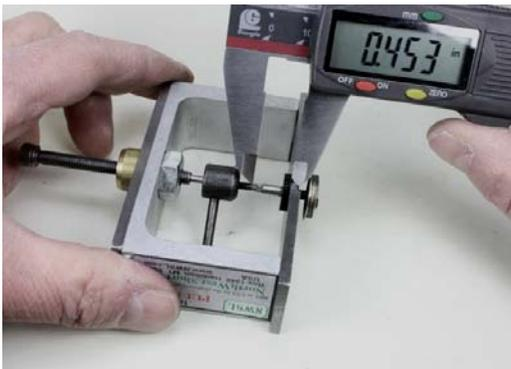
17. Insert the motor adjustment screw (forward screw removed in step 3) and snug it up. Apply power to the motor leads and advance this screw until you hear the motor rpm increase (mechanism seems to relax).
