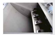
tangential cutting chamber paired with the open rotor design aggressive ensures reliable ingestion voluminous parts. The curved cutting chamber back-wall reduces the risk of parts getting stuck.
