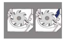
The easily removable deflector wedge acts as a third stator blade and can be used to adjust the aggressiveness of the rotor at the first cutting point.
