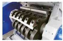
The specially angled rotor automatically pulls the fed pipes or profiles into the cutting chamber. This design also regulates the amount of material.
