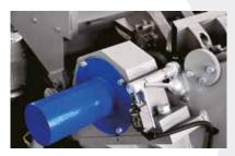
The heavy duty bearings are separated from the cutting chamber to avoid lubricants entering the cutting chamber and bearing failure due to material contamination in the bearings.
