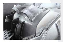
The combination of pre breakers and counter knives create a high impact powers resulting in a high degree of disintegration and high throughput rates.
