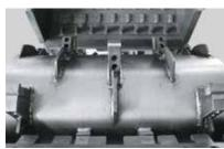
The ZHM hammer mill features a flat rotor with innovative welded tool holders. This heavy duty rotor design ensures a smooth operation on various materials.
