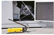
To ensure a safe operation and quick and easy access for cleaning and maintenance the GSC 500 machine's cutting chamber is opened hydraulically.
