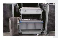
The user friendly design of the GSC series granulators allows quick and easy access to the cutting chamber for maintenance and cleaning.
