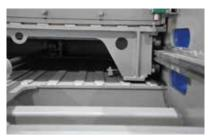
The ZCS system uses a sturdy roller guided drawer type ram to feed the material into the shredder. Segmented cutting chamber and ram allow trouble free processing of thin materials.
