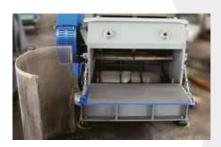
The user friendly design of the GSE series granulators allows quick and easy access to the cutting chamber for maintenance and cleaning.
