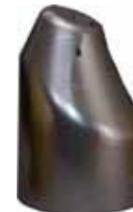
The slider eccentric bit is a cost effective solution for situations involving extreme washouts, ledging and doglegs. Through rotation provided by the casing landing tools, the long eccentric nose of the bit is aligned towards the open hole, acting as a guide to deflect off of the obstructions and continue past quickly. It features a smooth profile that excels at sliding, but is not designed for fill agitation. The Slider is made of aluminum composite, and is completely PDC drillable.
