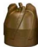
The Casing Pilot is a PDC drillable bit made completely out of bronze, with tungsten carbide cutting faces and tungsten buttons on the OD, helping to reduce wear through friction. The Casing Pilot was designed to be the best all-around bit, suitable for reaming and bridge removal regardless of geology. The profile of the Casing Pilot maintains a long taper, allowing for deflection off of ledges, washouts, and doglegs.
