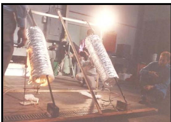
Figure 3 - UL181 Test Start
