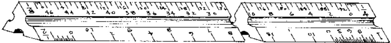
Illustration: Architect’s scale rule with twelve scales (four per side).
