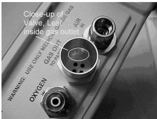
Location of Leaf Valve inside Adapter
