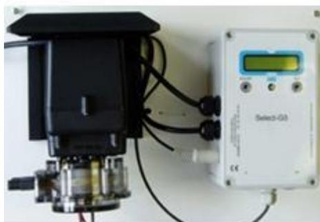
**Fig. 8: Water medication metering device**
