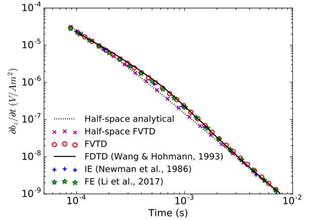
**Figure 3:** Different numerical results for the block model as calculated by FDTD (Wang & Hohmann, 1993), integral equations (IE) (Newman *et al.*, 1986), the FVTD method presented here, and FE (Li *et al.*, 2017) as well as the analytical and FVTD results of the half-space model.
