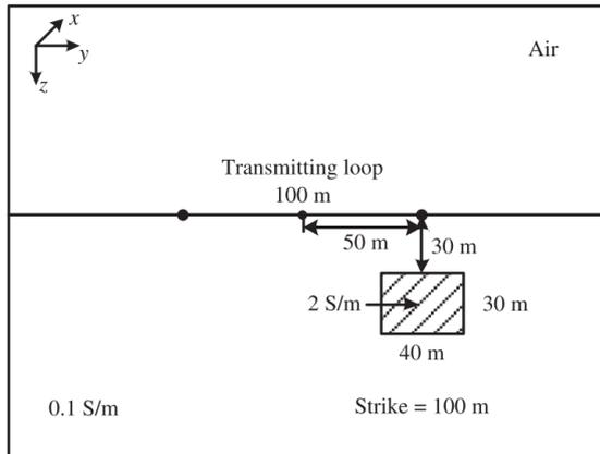
**Figure 2:** A section view of the 3D block model (Li *et al.*, 2017)
