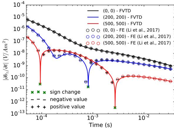
**Figure 5:** Numerical results of FVTD and FE methods for the same Ovoid Zone model. The observation locations (0, 0), (200, 200) and (500, 500) m are shown in Fig. 4 (the red points), which are relative to the loop center.
