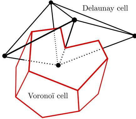
**Figure 1:** A dual mesh comprised of tetrahedral and Voronoi mesh. The circumcenters of the tetrahedra form the vertices of the Voronoi cells. The edges of the Delaunay (Voronoi) cells are orthogonal to the Voronoi (Delaunay) faces (Jahandari & Farquharson, 2014).
