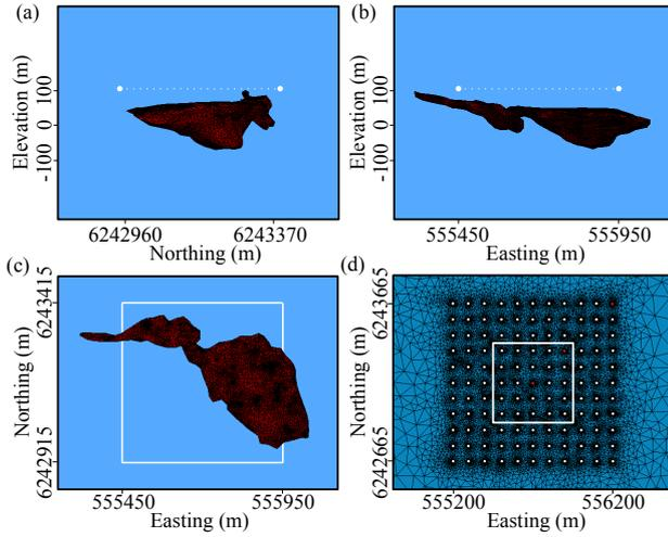
**Figure 4:** The mesh for the Ovoid Zone model. The white rectangle represents the loop wire. The white and red dots both inside and outside the loop wire are the locations of the observation points (Li et al., 2017).
