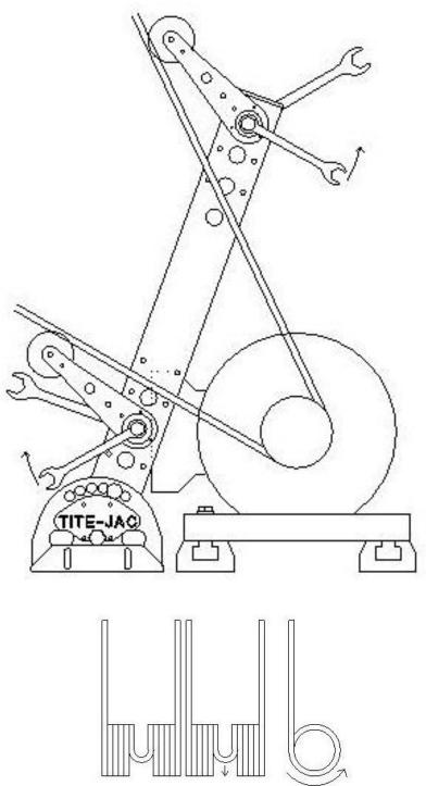
The spring tension must be adjusted in the direction indicated above. The spring must always wind tighter. If you tension the spring in the other direction the spring will start to unwind and fail prematurely. These springs are pickup tines from a New Holland combine and can be purchased at any agricultural implement dealer.
