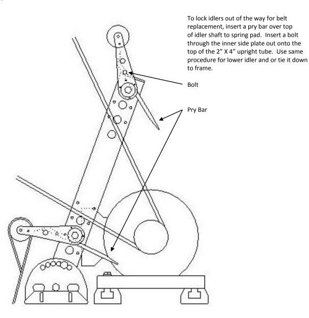
If you are unable to insert a bolt into tube to hold bottom idler away from belt use a rope or chain to tie it down to frame rail.
