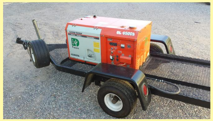
This 6,500 watt single phase generator is diesel powered and mounted on a small 2 wheel trailer with a 2" hitch for easy towing. It has the convenience of a very low profile so it is easy to hide from view. It is an extremely quiet running unit powered by an economical Kubota diesel engine.
