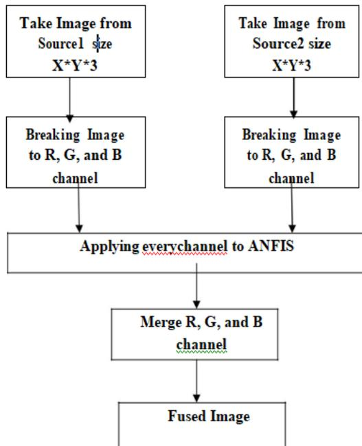
**Figure4: Work Flow Diagram of Image Fusion using Adaptive Neuro Fuzzy**
