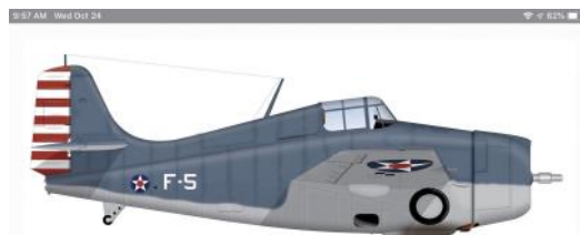
The change to the Blue-Gray over Light Gray paint scheme is illustrated in this profile of an F4F-3A assigned to VF-2 in early 1942. The 2 has been deleted from the fuselage code, and the red and white stripes, intended to be an identification aid for American aircraft, have been added to the rudder. Note the demarcation line between the Blue-Gray and Light Gray on the forward fuselage. It is about even with the leading edge of the wings. This was fairly standard on F4F-3s and F4F-3As, although there were some variations, particularly on those aircraft repainted at the squadron level. This would later be changed on F4F-4s. (Artwork by Rock Rozsak)
