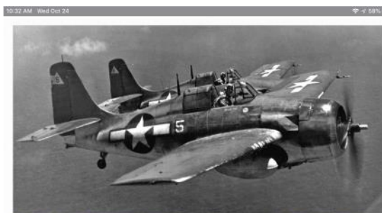
Two FM-2s from USS WHITE PLAINS, CVE-66, fly in tight formation on June 24, 1944. Both Wildcats are painted in the tri-color scheme. Note that aircraft number 5 has the aft end of the antenna wire attached to the mast at the top of the rudder, but number 11 has the later and more common arrangement with the aft end of the wire attached to the leading edge of the vertical tail. (National Archives via Bell)
