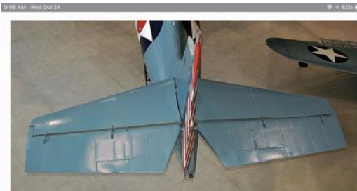
The horizontal tail was a conventional design with metal covered horizontal stabilizers and fabric covered elevators. Metal trim tabs were on both elevators, and the actuator for the one on the right was on top, while the actuator for the one on the left was on the lower surface. This was because the horizontal stabilizers and elevators could be fitted to either side of the aircraft. The inboard edge of each elevator was tapered to provide sufficient clearance for the movement of the rudder. (Kinzey)
