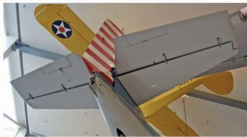
An underside view of the horizontal tail provides a good look at the metal trim tabs and the four hinges for the elevators. An inspection panel is located just forward of the trim tab on the left elevator, just as an identical panel was located forward of the trim tab for the right elevator on the upper surface. (Kinzey)
