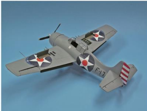
All of the Trumpeter 1/32nd scale Wildcats have parts to build the gun bays in the open position, revealing the guns and ammunition boxes inside. These features are visible on this late F4F-3 built by Bob Bartolacci. (Bartolacci)
