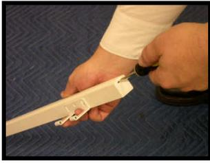
Insert screwdriver into slot under filler strip.
