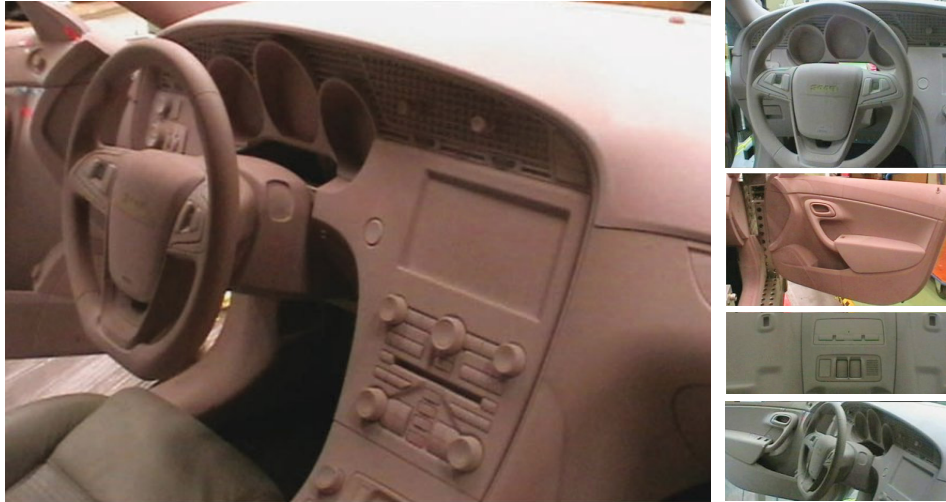
Production of interior cubing parts for a passenger car cabin with RAKU-TOOL® MB-0720 board material.
