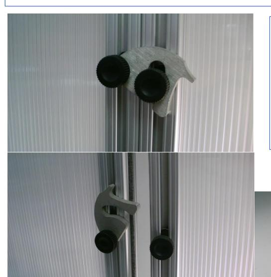
Our camlocks consist of an aluminum body with a radial slot that is not concentric to its pivot point. The farther you push, the tighter it squeezes the panels together. We implement thumb screws and t-nuts to make the installation very simple without the use of tools. The picture to the left shows how we machine slots into the extruded panel frames to allow for a quick installation of the camlock assembly.
