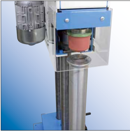
Example for utilization of the large working area: Printing on the face of a cylinder
