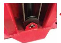
3/8"/ 76mm non fatigue equalization cables and 5" / 127mm steel pulleys
