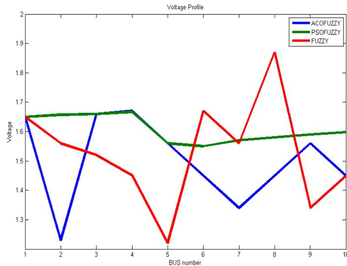
Fig.6: Voltage profile comparison of different Algorithms.
