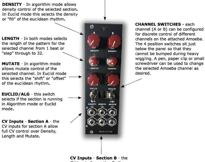
CV Inputs - Section B - the CV inputs for section B allow full CV control over Density, Length and Mutate.
