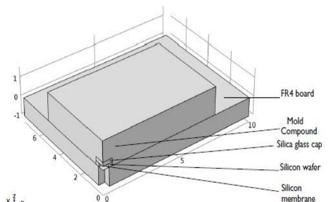
Figure 1: Component Geometry
