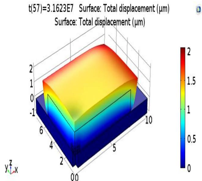
Figure 7: Displacement after 1 year in Polyurethane
