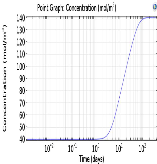
Figure 4: Moisture concentration at die location over time for Polyurethane
