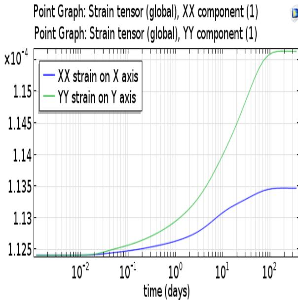
Figure 8: Evolution of measured strain on membrane axes Polyurethane
