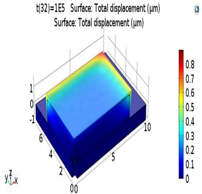
Figure 6: Displacement after 2 days in Polyurethane
