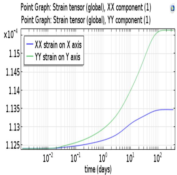
Figure 14: Evolution of measured strain on membrane axes Polyimide
