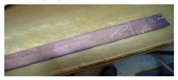
It is very important that all angles at the blade tang junction be square 90deg. angles. At the tang blade junction the tang is undercut slightly to allow thread tapping all the way down to the blade.
