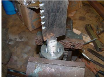
Next the handle is threaded. It is very important that the tap be square in the handle tubing. Also that the ends of the tubing are square. Failure to square the ends of the tubing and squaring the tap will result in an improper fit to the guard.
