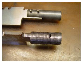
Next the threaded rod is squared to the shoulders and 2 guide pin holes are drilled threw the threaded rod and the tang. I used a 3/32 drill and secured the threaded rod with 3/32 Stainless pins. Note that the pins must not extend out into the threads of the rod.
