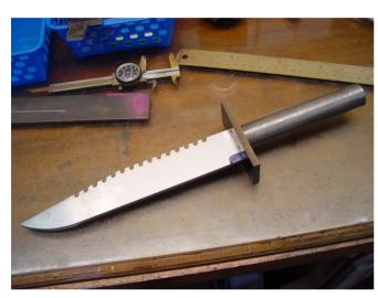
For the handle tubing I used 11/16 ID 4140 with a 1" OD. Once the handle is tapped, and the guard is slotted you can do a test fit.
