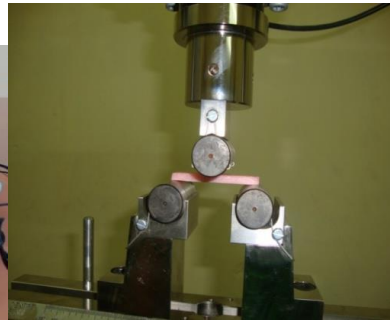
Fig 11: Samples evaluated for fracture resistance using UTM
