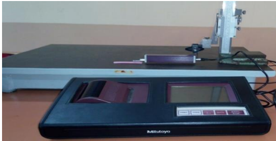
Fig 10: Samples evaluated for surface roughness using profilometer
