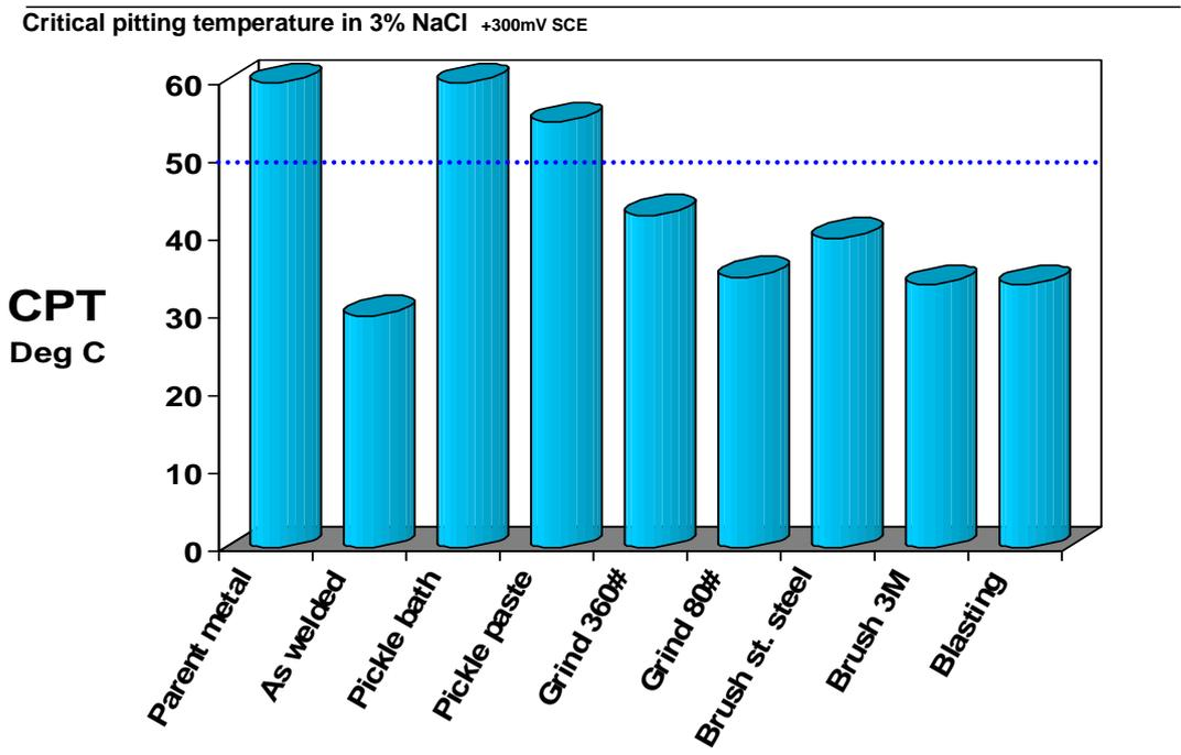
Figure 1. The effect of various mechanical and chemical cleaning methods on the pitting resistance of SAF2205 duplex stainless steel.
