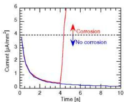
Fig. 4. Corrosion current at the reference potential
