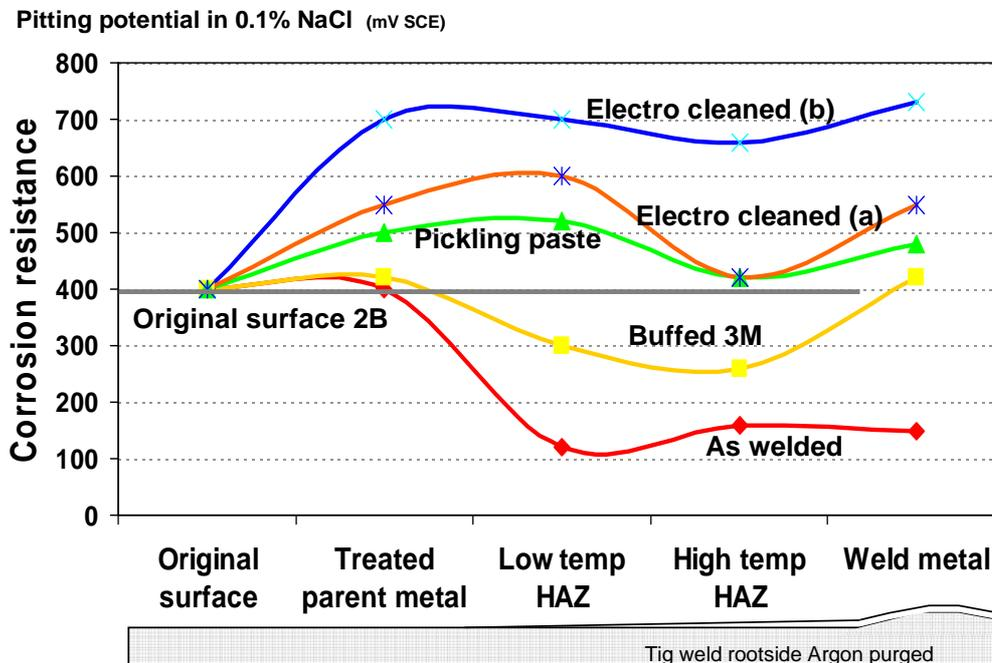
Figure 5. Effect of cleaning methods on a stainless steel weldment.
