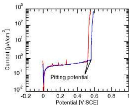
Fig. 3. Calibration scan determines pitting potential
