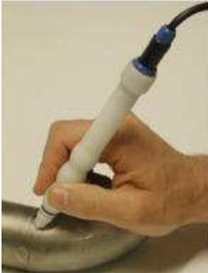
The sensor makes electrolytic contact with the surface. Capillary forces cause electrolyte flow through a porous polymer pen.
