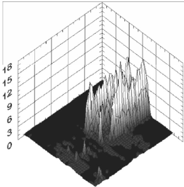
Fig. 8: Potentiostatic current [ $\mu\text{A}$ ] distribution on a weld on DIN 1.4301 at 0.3 V SCE in 0.1 M NaCl over an area of 30 x30 mm. The lower left side of the sample has been electrocleaned showing passive behavior, while the non treated upper right side shows pit initiation along the weld. (4)
