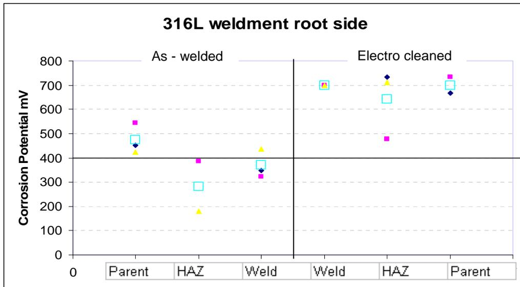
Figure 6. Showing the positive effect of electrocleaning on the root side of a weldment.
