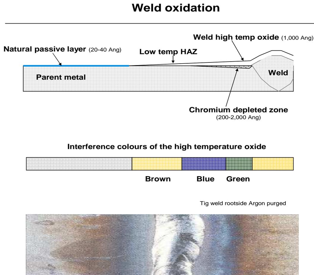
Figure 2. Surface oxidation, depleted zone and interference colours of stainless steel welds.
