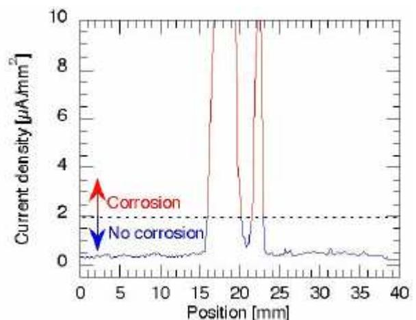
Fig. 7: Potentiostatic line scan (4) over a weld of a stainless steel (DIN1.4301) showing the variation in corrosion current of a 40mm test length. Tested in 0.1 M NaCl at 260 mVSCE.
