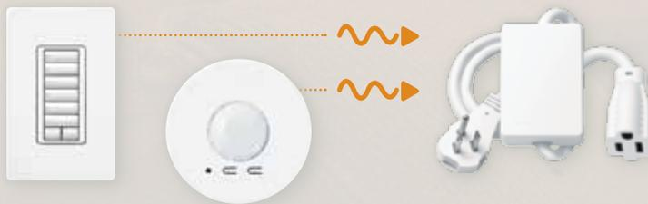
**How it works:** The plug-in appliance module receives a radio frequency signal from a keypad or sensor “telling” it to turn off standby power when the appliance isn't being used.
