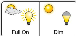
Daylight sensors automatically dim the lights when there's sufficient daylight
