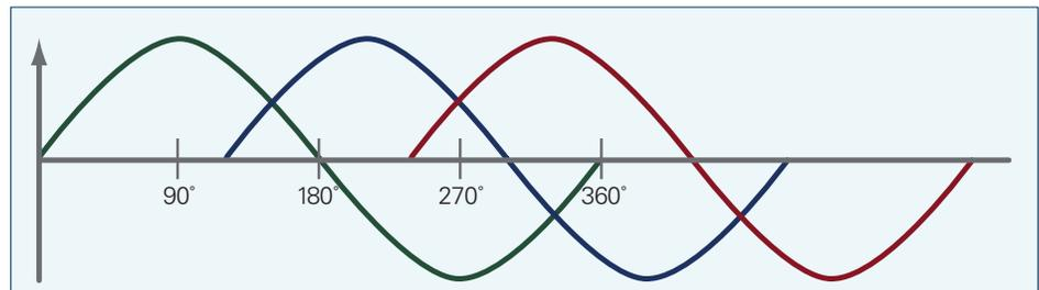
Figure 1. Three-phase power
