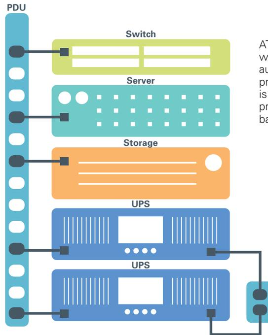
ATSs provide power redundancy to equipment with only one power supply. The ATS automatically transfers the power from a primary source to a secondary source if there is a problem with the primary. Once the primary source is restored, power transfers back through it.
