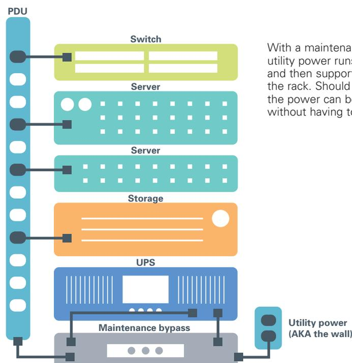
With a maintenance bypass (MBP) for example, utility power runs through the MBP via the UPS and then supports the rest of the equipment in the rack. Should the UPS need to be replaced, the power can be switched away from the UPS without having to shut down your equipment.
