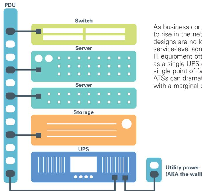
As business continuity requirements continue to rise in the network closet, traditional power designs are no longer adequate to meet IT service-level agreements. However, single-corded IT equipment often complicates system design, as a single UPS or rack PDU may represent a single point of failure. Maintenance bypass or ATs can dramatically improve system reliability with a marginal cost impact.
