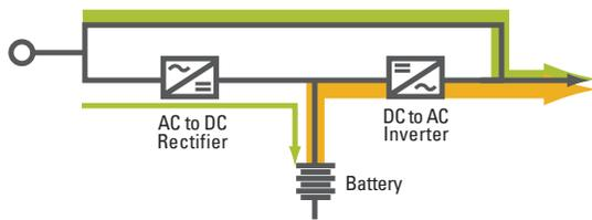
**Line-interactive UPSs** actively regulate voltage either by boosting or decreasing utility power as necessary before allowing it to pass to the protected equipment or by resorting to battery power. Line-interactive models are ideal for applications where protection from power anomalies is required, but the utility power is relatively clean. MDF and IDF communication closets, non-centralized server and network rooms, and general IT enclosures are ideally suited for this topology.
