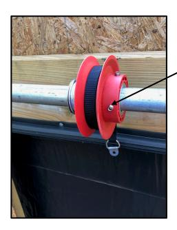
Set Screws must Be on Right side when installed
