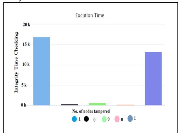
Above graph shows on X-axis No. of fragment tempered and On Y-axis Time to check integrity of each file (ms).The graph is get by TPA After checking each file integrity. After checking integrity tempered nodes fragment is replaced by replica of that fragment here attack is detected and prevented so user can get original file that is uploaded by owner.
