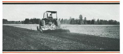
moldboard plow, the ROTASPIKE rounds out a total tillage program. It promotes moisture retention and erosion control for all types of seedbeds. The spike rotor is particularly suited to deep seedbeds like potatoes, because it breaks and crumbles the clods to the full tillage depth of 7 inches. The full-width crumble roller accurately controls depth while firming and leveling the seedbed and eliminating wheel marks.
