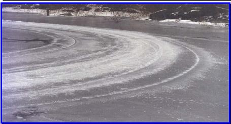
Using the sled with the wear rods in poor condition, we were able to sustain approximately 6 mph on this skid pad. Utilizing the sled with the carbides, we were able to sustain 16 mph. The following graphs illustrate the lateral G-forces attained in the lateral skid pad
