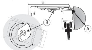
Standard, heavy duty, ceiling mount and double mount installations use the same mounting clip (93630) and rods attach the same way.
