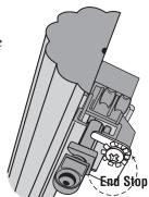
Remove any extra carriers and capture end most carrier with End Stop to lock remaining carriers within track. Tighten End Stop Screw to lock carriers in track.
