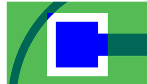
Solder paste wicking Maximum exposed etch in soldermask
