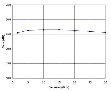
Figure 1: RFM1.6-30-500XR Typical Gain @ Pout = 500W.
