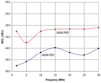
Figure 2: RFM1.6-30-500XR Typical IMD<sub>3</sub> @  $\Delta f$ =10kHz, 500W PEP and 400W PEP.
