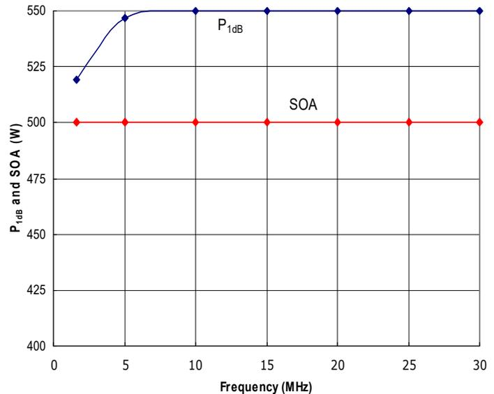
Figure 4: RFM1.6-30-500XR Typical P<sub>1dB</sub> and Safe Operating Area (SOA). **Do not exceed the SOA shown above without first contacting RFMPT to discuss your application.**
