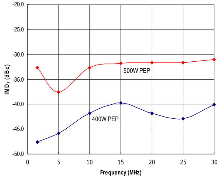
Figure 2: RFM1.6-30-500XR Typical IMD<sub>3</sub> @ Δf=10kHz, 500W PEP and 400W PEP.
