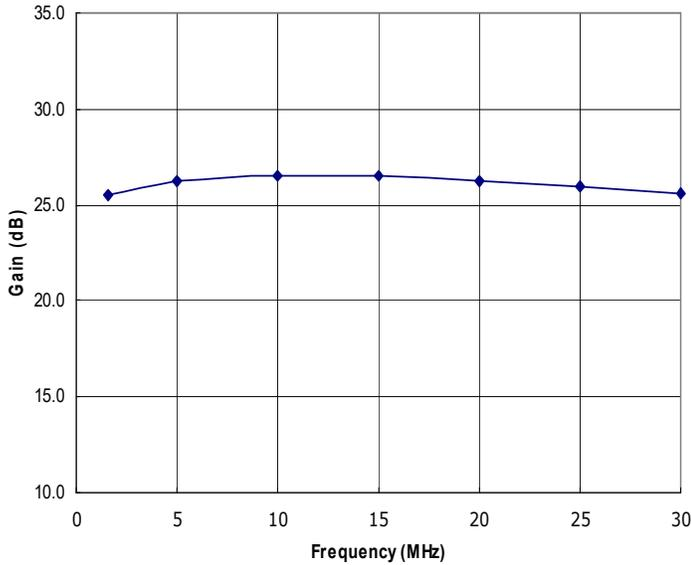
Figure 1: RFM1.6-30-500XR Typical Gain @ P<sub>out</sub> = 500W.
