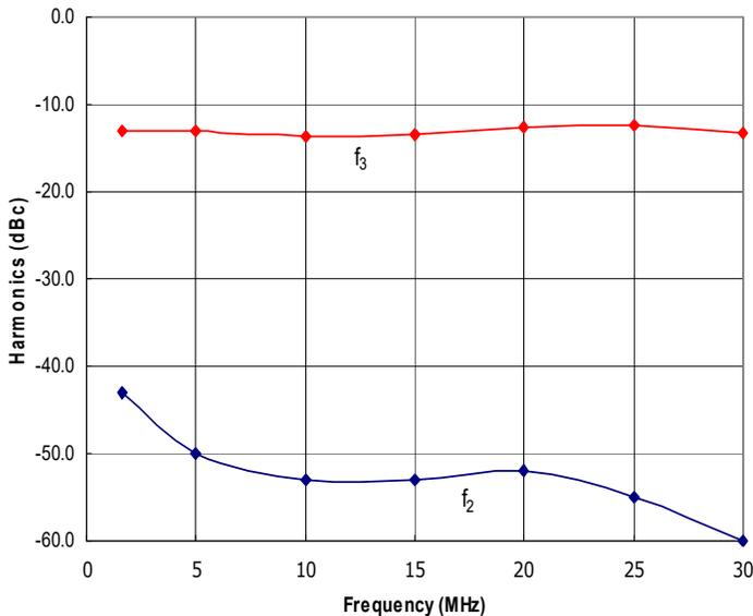
Figure 3: RFM1.6-30-500XR Typical f<sub>2</sub> and f<sub>3</sub> @ P<sub>out</sub> = 500W.
