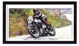
cornered race in which Daniell pushed the lap record up to 90.99 mph he won the race by 15 seconds at an average speed of 89.11 mph. The Norton has a single cylinder, single port, overhead twin camshaft engine which is carried in a special spring frame with telescopic front forks.
