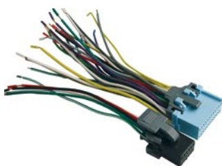
FD-5521-1M FORD / LINCOLN / MERCURY 03-UP (male plug) • Plugs into Factory Radio S # H623
