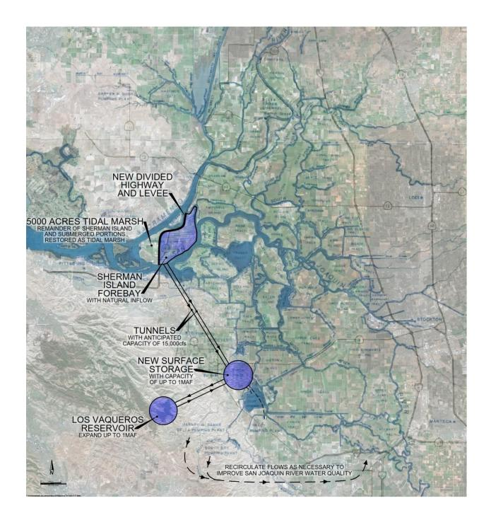
**Schematic of the Western Delta Intakes Concept**
