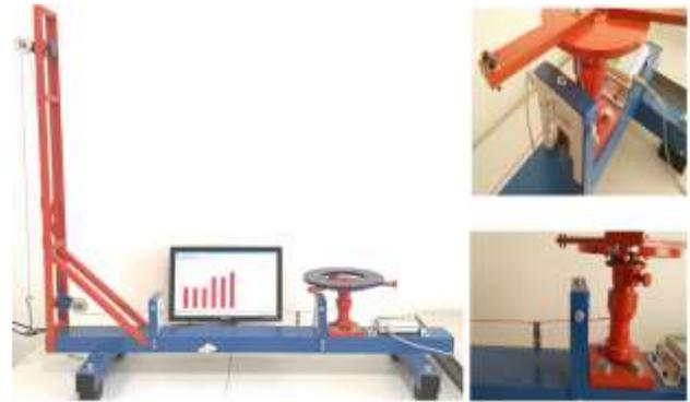
Figure 6. Moment of inertia apparatus set-up with computer interface
