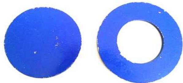
Figure 7. Moment of inertia specimens
