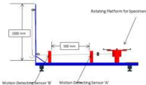
Figure 2. 2-D assembled view of mass moment of inertia test rig
