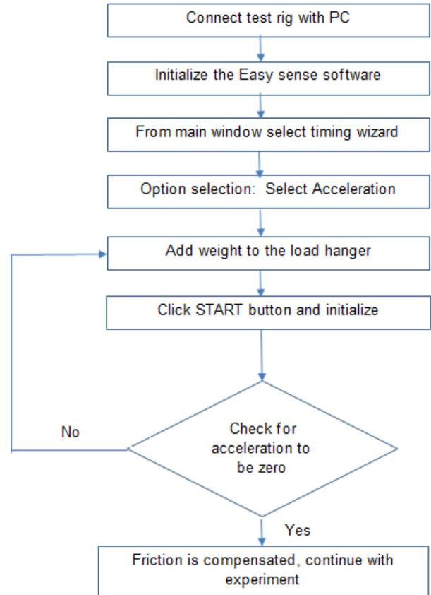
Figure 3. Flow diagram for software interface
