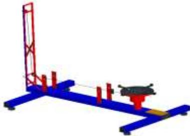
Figure 1. 3-D assembled view of mass moment of inertia test rig
