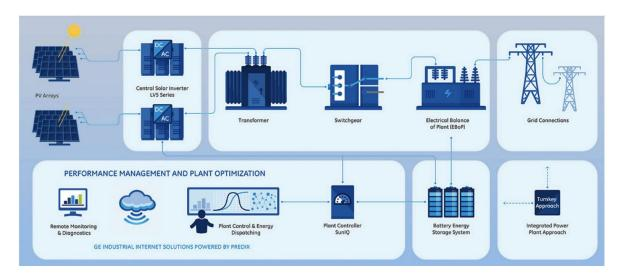
Notice all that power conversion equipment in the top row: inverters (DC to AC), transformers, switchgears, electrical balance of plant, plus battery energy storage systems in row 2. All this apparatus makes noise. Complicated noise.
