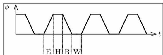
Figure 1. Trapezoidal four-phase power clock
