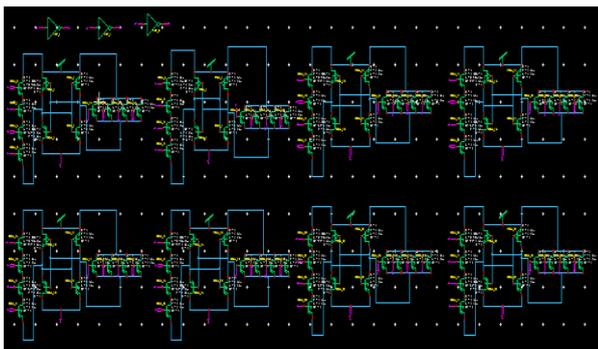
Figure 24.PFAL 1\*8 Demultiplexer Schematic Design
