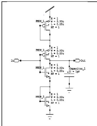
Figure 7.Basic Proposed Logic Inverter Schematic
