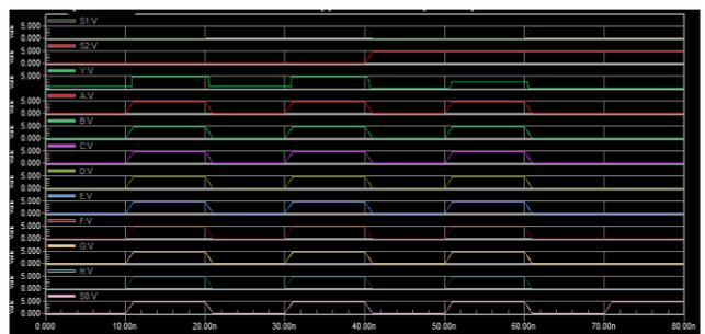
Figure 11.ECRL 8\*1 Multiplexer Output Waveform
