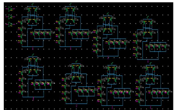
Figure 22.2N2N2P 1\*8 Demultiplexer Schematic Design
