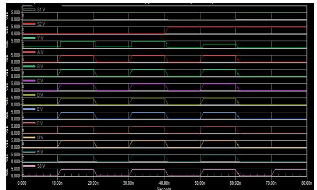
Figure 15.PFAL 8\*1 Multiplexer Output Waveform
