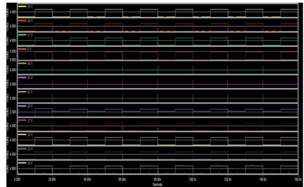
Figure 21.ECRL 1\*8 Demultiplexer Output Waveform
