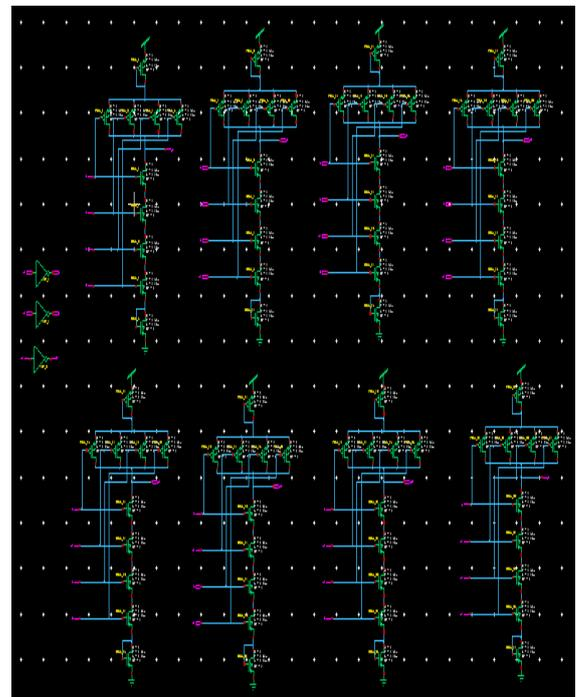
Figure 26.Proposed Logic Circuit 1\*8 Demultiplexer Schematic Design
