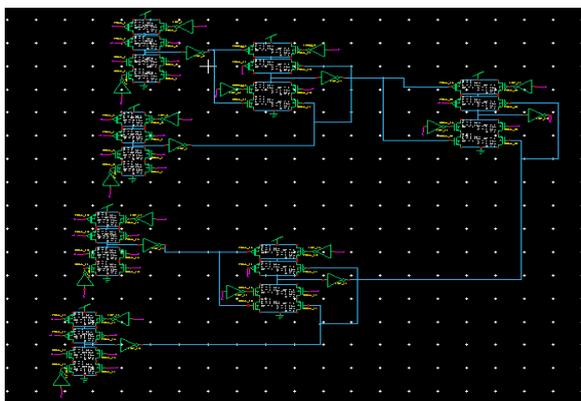
Figure 8.CMOS 8\*1 Multiplexer Schematic Design
