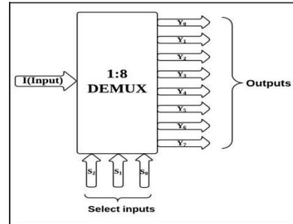
Figure 6. Block diagram of 1\*8 Demultiplexer
