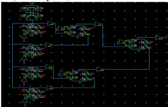
Figure 14.PFAL 8\*1 Multiplexer Schematic Design
