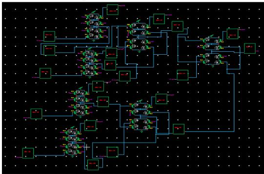
Figure 12.2N2N2P 8\*1 Multiplexer Schematic Design
