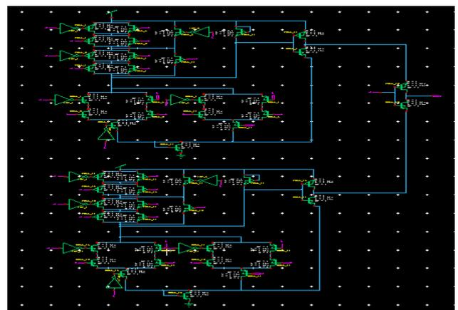
Figure 10.ECRL 8\*1 Multiplexer Schematic Design
