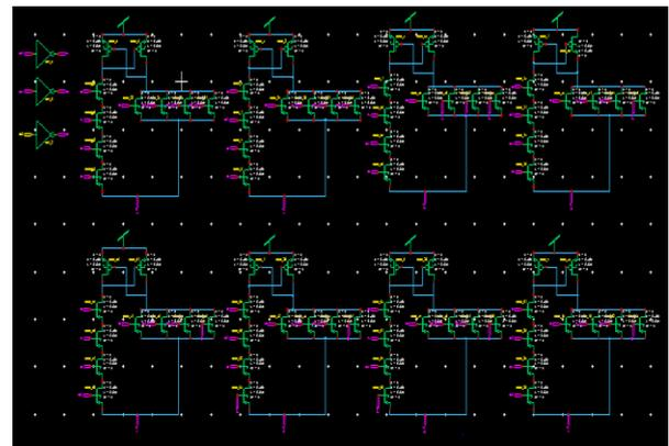
Figure 20.ECRL 1\*8 Demultiplexer Schematic Design
