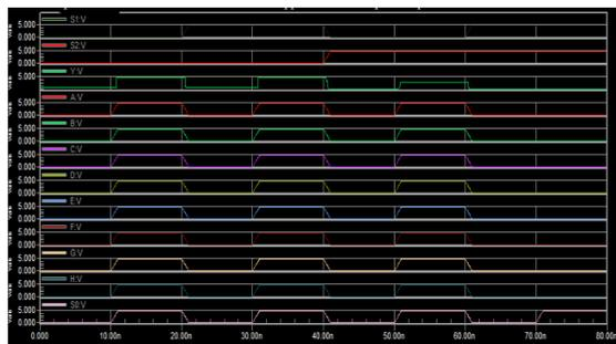
Figure 13.2N2N2P 8\*1 Multiplexer Output Waveform
