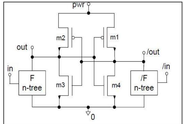
Figure 3. 2N2N2P General Schematic
