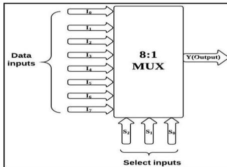
Figure 5. Block Diagram of 8\*1 Multiplexer
