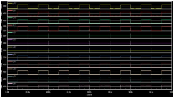
Figure 23.2N2N2P 1\*8 Demultiplexer Output Waveform
