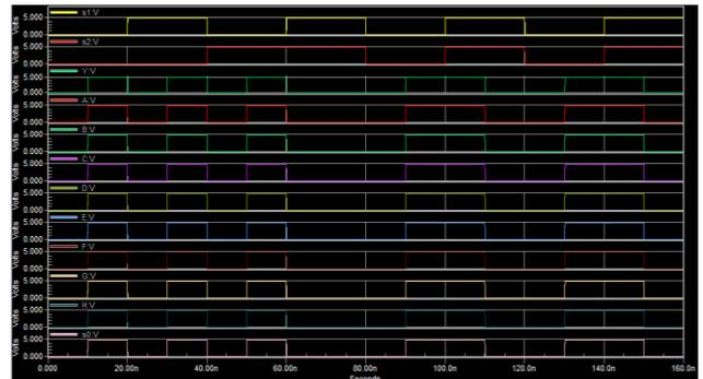
Figure 9.CMOS 8\*1 Multiplexer Output Waveform
