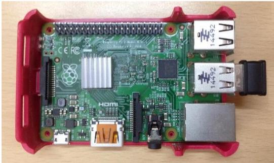
Fig.4: Raspberry Pi 2 Module
