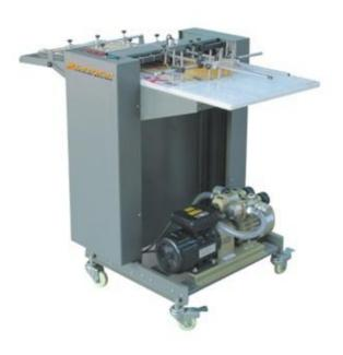
Shark Finishing Machinery introduces to its line of digital print finishing equipment the SF-25 Automatic, Air Feed, universal Paper Feeder. This stylish, heavy duty paper feeder is easy to use and is equipped with an adjustable delivery table, variable speed and heavy duty locking casters. It has a maximum paper size of 25.5 inches wide x 31.5 inches long and a minimum paper size of 8.25 inches wide x 6 inches long.
