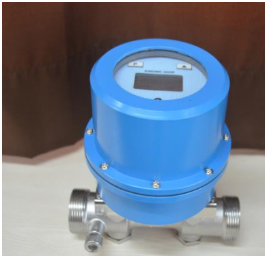
Fig.6: Ultrasonic Flow meter
