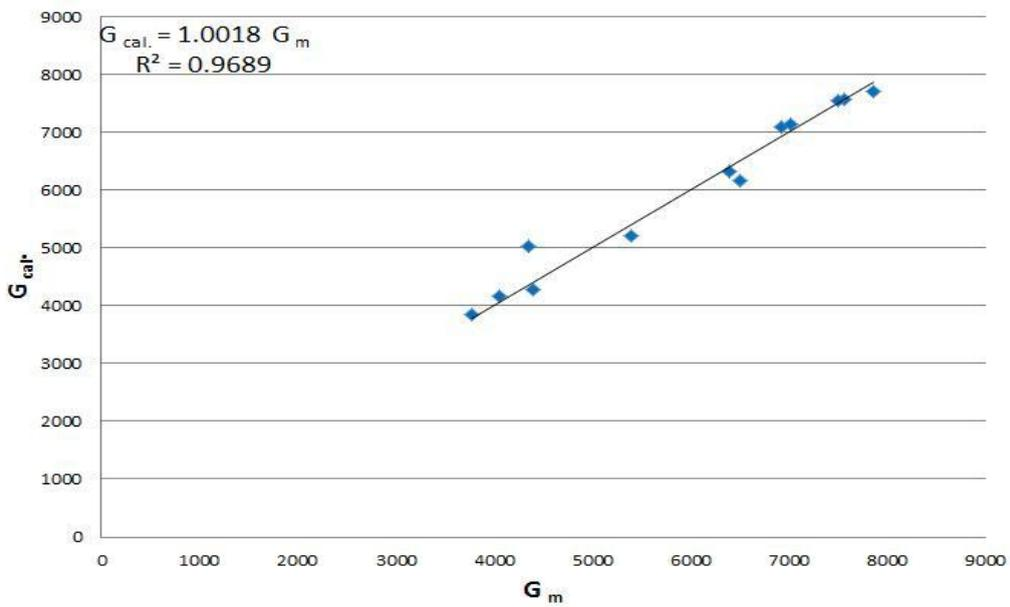
Fig. 3: Comparison between measured ( $G_m$ ) and calculated ( $G_c$ ) global solar radiation values for monthly average data through the study period at Qena.
