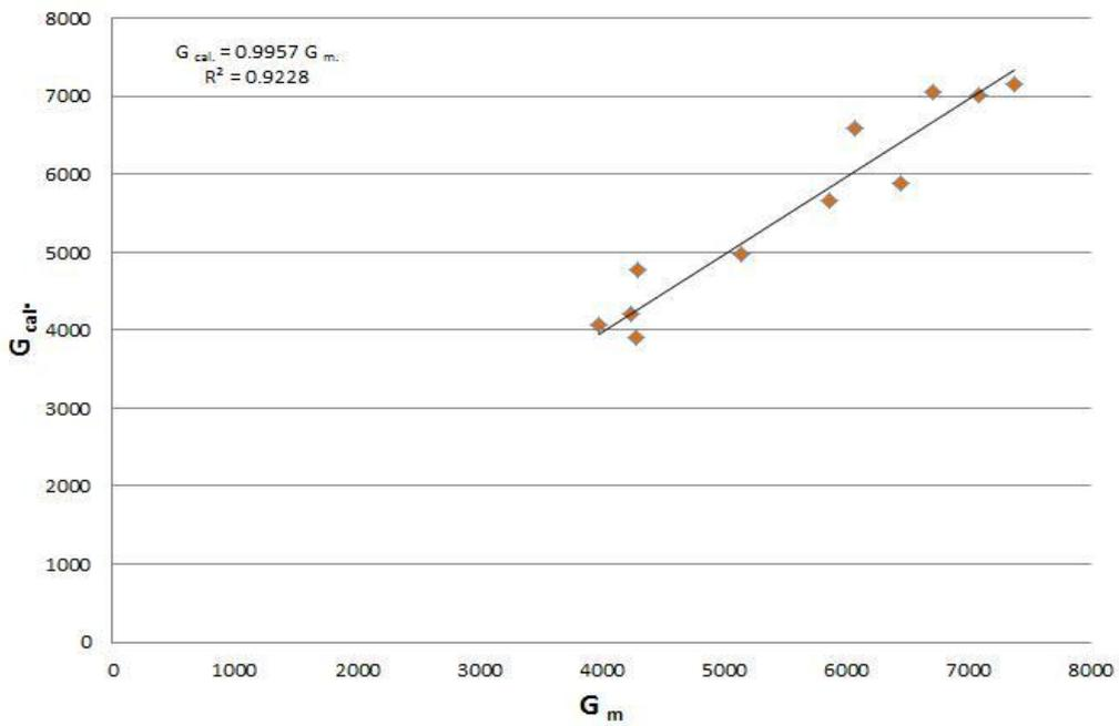
Fig. 2: Comparison between measured ( $G_m$ ) and calculated ( $G_c$ ) global solar radiation values for monthly average data through the study period at Mars Matrouh.
