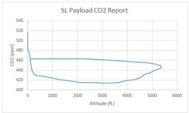
As shown by the graph, the CO2 levels stay constant at about 460 ppm during ascension until after apogee, where it drops down to almost 410 ppm and spikes back up when the rocket landed.
