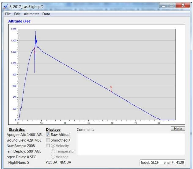
Judging by the altitude spikes of the extremely low apogee, the avionics facing the drogue chute may not have been properly insulated. That is not the case for the avionics facing the main chute, as there is no observable spike in altitude.
